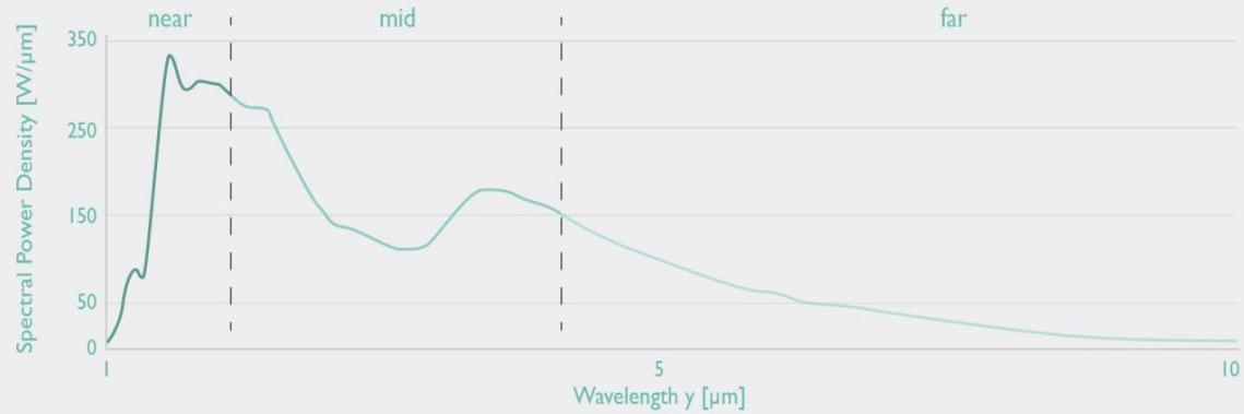
Measuring Front emission with reflector. Total power consumption 500W Percentage of radiation from the front emitter = 98.6%
